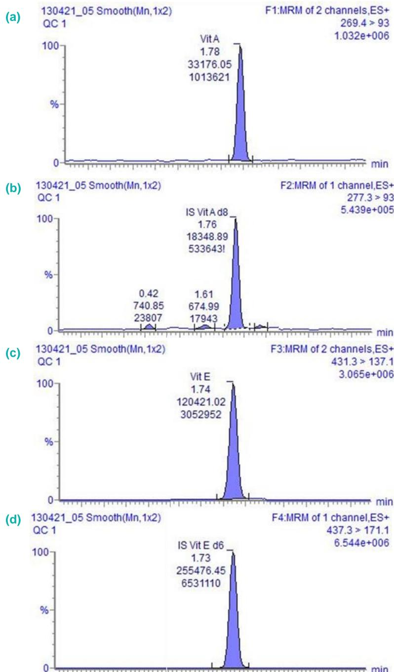
Figure 1 - Typical chromatograms: (a) Retinol quantifier ion, (b) Retinol-d8 IS, (c) alpha-tocopherol quantifier ion, (d) Alpha-tocopherol-d6 IS
