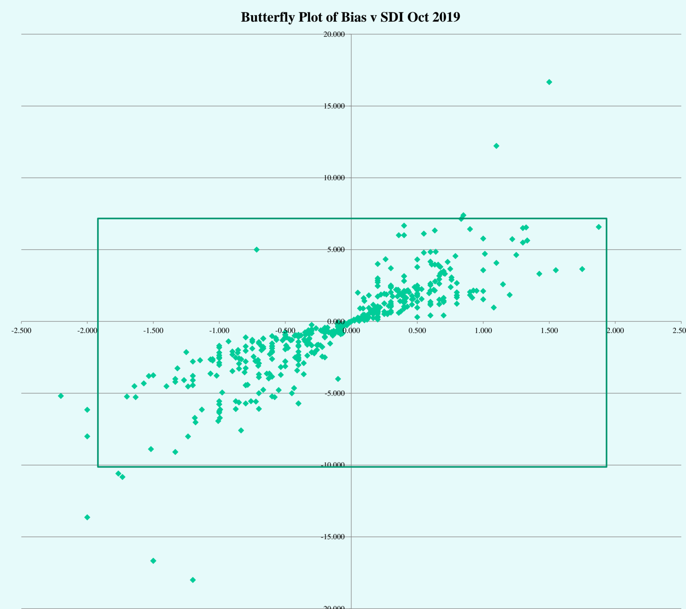
Fig 3 showing a plot of combined SDI & bias data. Each green dot is a single analyte. Ideally, all dots would be within the box. The dimensions of the box can be altered to appropriate targets for different analytes, eg. using NQAAP targets. Analytes outwith the box would require to be investigated
